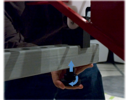
Non-stinger method to mount Model 3142E to 7-TR
